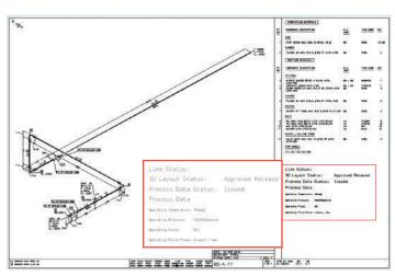
Linked engineering data can be referenced and used on schematic and 3D deliverables. The example shows process data from AVEVA Engineering included on a piping isometric drawing.
